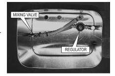
sure". It is not the primary adjustment for the brix level. From our testing, it has been shown that exact PSI on the gage does not directly correlate to a brix level from unit to unit and from installation location to installation location.
